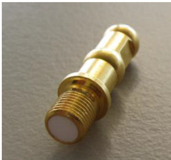
Fig. 140: DiTi cone with inline filter
